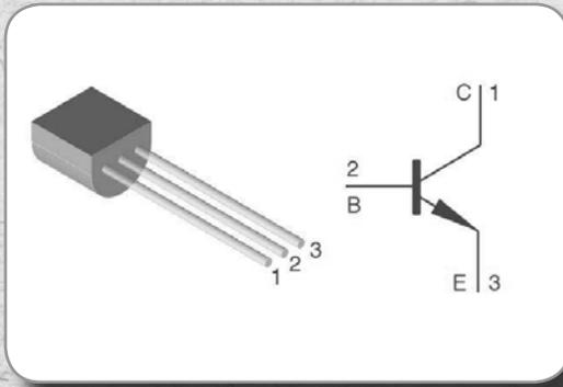
Figure 10.9: Pin configuration of the BC548 transistor (Source: Vishay data sheet)
