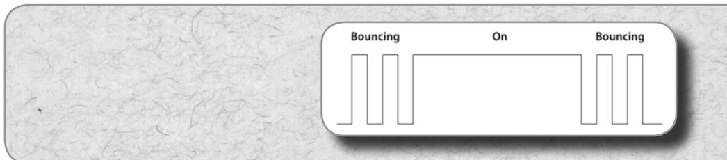
*Figure 10.5: This is the impression the microcontroller gains at the digital input due to the bouncing effect of a button*
