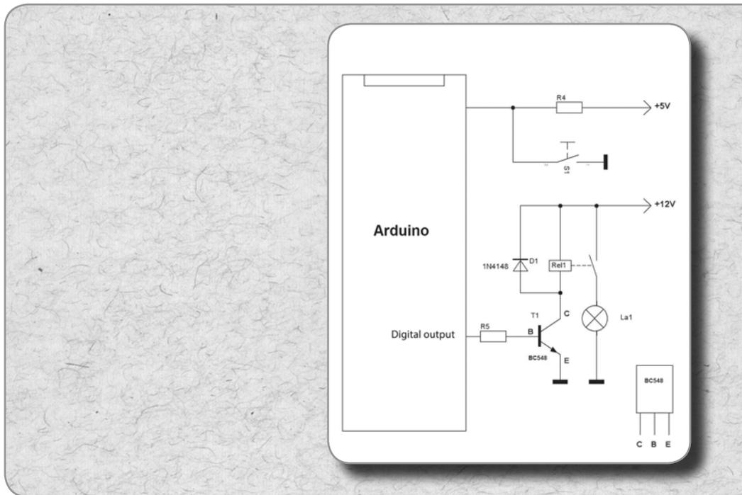
Figure 10.10: Relay at the digital pin of the Arduino
