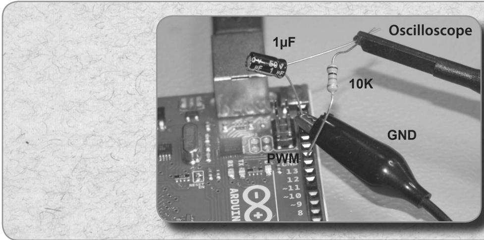
Figure 10.3: Set-up of the RC circuit. The resistor is connected to analog output 11 on the Arduino board. The negative terminal of the capacitor is attached to ground. This circuit filters the PWM signal so that only the envelope of the sine function is visible on the oscilloscope.
