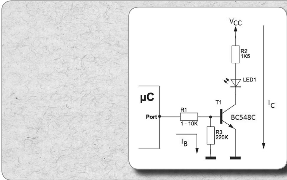
Figure 10.8: A transistor at the digital output of the Arduino microcontroller ( $\mu\text{C}$ );  $I_B$  = base current,  $I_C$  = collector current. Both base and collector current flow through the emitter. The tutorial kit contains low-current LEDs ( $I_{\text{forward}} = 2 \text{ mA}$ ), hence the large  $1.5 \text{ k}\Omega$  series resistor R2.
