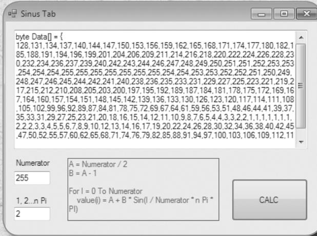
Figure 10.2: The program Sinus Tab that calculates the values of the sine wave table
