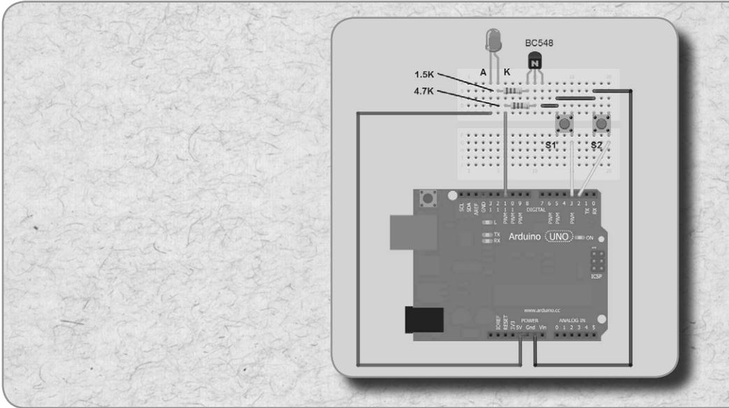
Figure 10.1: Diagram of the set-up for an LED dimmer with transistor
